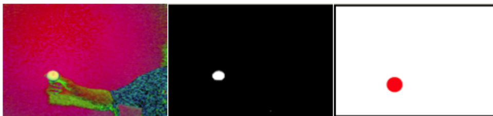
Figure 7.1: (a) a view in HSV color space, (b) a binary image in which the red ball is isolated, (c) simulated version of red ball
