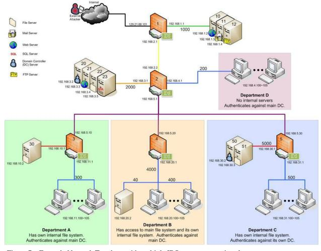
Figure 7 – Example Network Topology with multiple IDS on route to various hosts. Figure courtesy of Dr. Jay Yang
