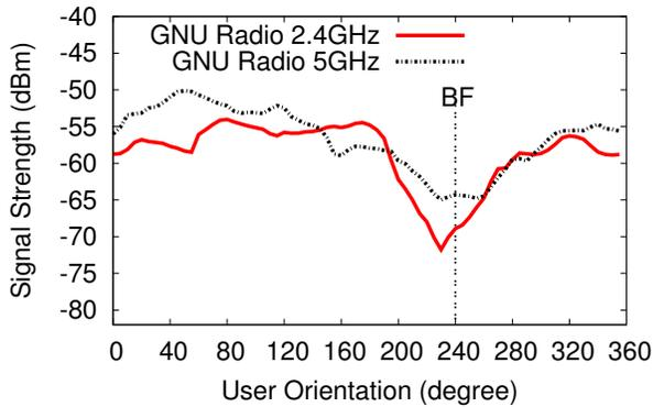
**Figure 11: Sample signal strength profiles as a user rotates, measured using USRP2 GNU radios operating on 2.4GHz and 5GHz. We observe the same signal-blocking artifact. As before, BF marks the direction where the user has her back facing the AP.**
