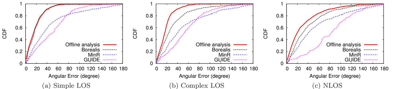
**Figure 8: Comparing Borealis to Offline Analysis, MinR, and GUIDE in the three environments.** Borealis significantly outperforms MinR and GUIDE, and is within a small distance from its offline version (Offline Analysis).
