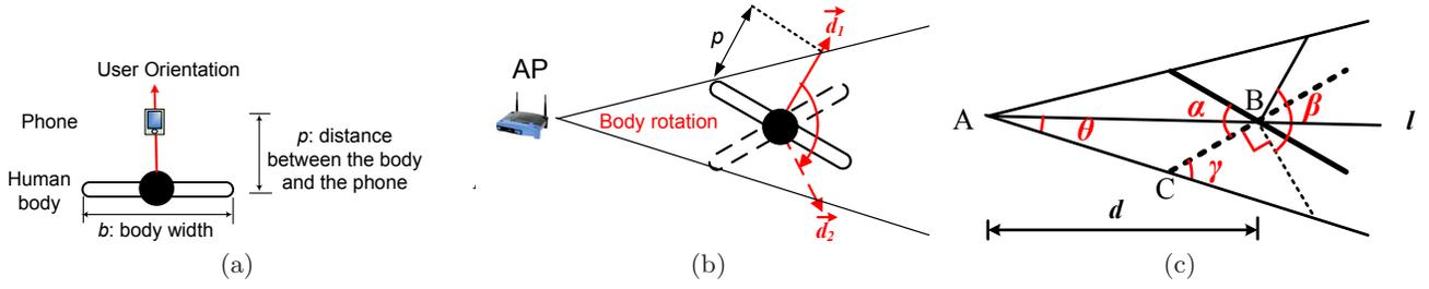
**Figure 4: An abstract model of the human shield effect.** (a) A simple model of a user holding a smartphone, with body width  $b$  and phone/body distance  $p$ . (b) The signal propagation condition as the user rotates. When the user orientation is between  $\vec{d}_1$  and  $\vec{d}_2$ , the LOS path will be blocked by the human body. This range of orientation is referred to as the blocking sector. (c) A geometric representation of the blocking sector.
