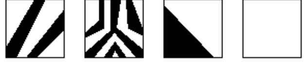
Figure 2: Different texture characteristics. From left to right, Flow, 2D pattern, Edge and Low Contrast.
