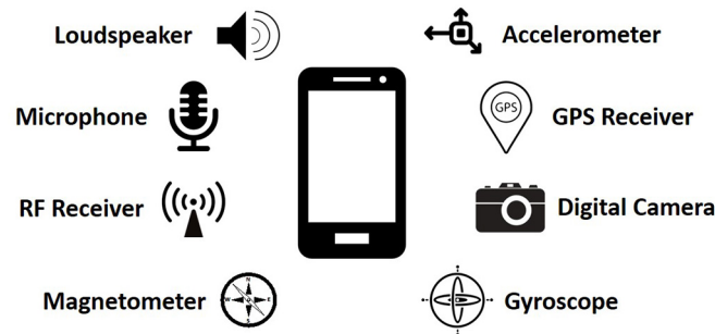
Figure 2.1. Sensors in a smartphone
