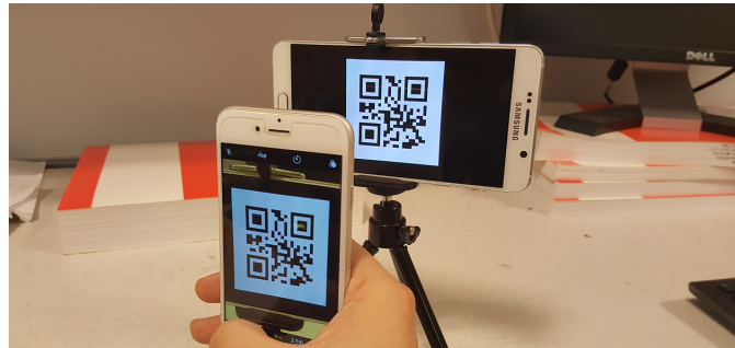
Figure 3.4. Use case: a user captures an image shown on the verifier's interface to be authenticated (or registered).
