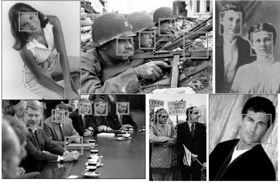
Figure 11: Some face detection results tested on the CMU frontal and profile image dataset.
