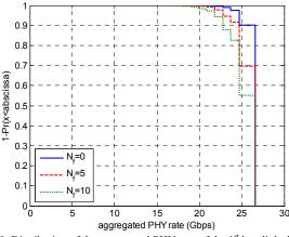
Fig. 10. Distribution of the aggregated PHY rate of the  $1^{st}$  hop links between the stations and the 60 GHz APs for the two-hop mesh (all the stations and the APs using the 6x6 square array antenna)
