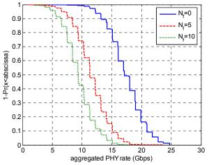
Fig. 16. Distribution of the aggregated PHY rate of the  $1^{st}$  hop links between the stations and the 60 GHz APs for the two-hop mesh (the stations with 4x4 square array antenna and the APs with 6x6 square array antenna)
