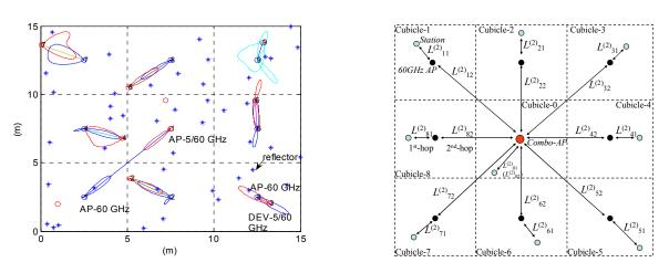
(a) 9-cubicle network topology with 5 reflectors/cell
