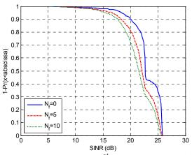
Fig. 8. Distribution of the SINR of the  $2^{nd}$  hop links between one of the 60 GHz AP and the combo-AP for the two-hop mesh (all the APs using the 6x6 square array antenna)
