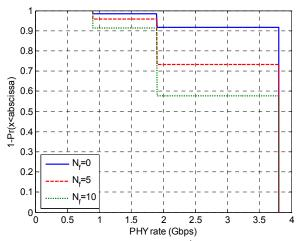
Fig. 15. Distribution of the PHY rate of the 2<sup>nd</sup> hop link between one of the 60 GHz AP and the combo-AP for the two-hop mesh (all the APs using the 6x6 square array antenna)
