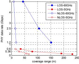
Fig. 1. Comparison of transmission ranges and data rates of 5 GHz and 60 GHz in LOS and NLOS environments using maximum transmit power per antenna ( $P_t = 24$  dBm for 5 GHz and  $P_t = 4$  dBm for 60 GHz)
