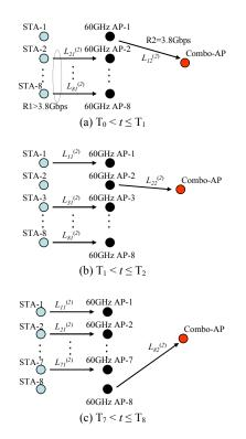
Fig. 11. Illustration of the two-hop mesh operation over the time  $T_0 < t \le T_8$  achieving the end-to-end throughput close to the maximum PHY rate of the 2<sup>nd</sup>-hop link
