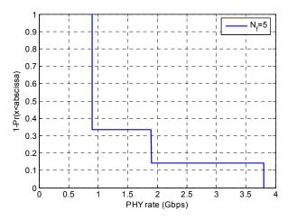
Fig. 17. Distribution of the PHY rate of one-hop link between one of the stations and the 60 GHz AP (the stations with 4x4 square array antenna and the APs with 6x6 square array antenna)
