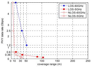
Fig. 2. Comparison of transmission ranges and data rates of 5 GHz and 60 GHz in LOS and NLOS environments using typical transmit power ( $P_t$  = 17 dBm for 5 GHz and  $P_t$  = -5.6 dBm for 60 GHz)
