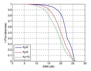
Fig. 14. Distribution of the SINR of the 2<sup>nd</sup>-hop link between one of the 60 GHz AP and the combo-AP for the two-hop mesh (all the APs using the 6x6 square array antenna)
