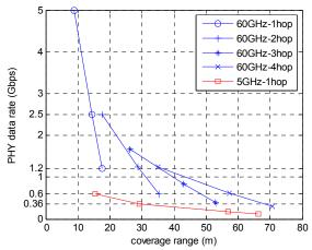
Fig. 4. Comparison of transmission ranges and data rates of 60 GHz multihop mesh and a single hop 5 GHz for NLOS environments using maximum transmit power per antenna
