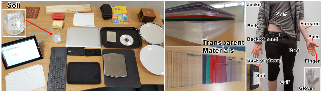
Figure 1. (left) The 26 materials/objects (including air and water) that we evaluate in the first study. (middle) 16 Transparent materials used in the second study, arranged from top to bottom according to the list in Figure 6. (right) 10 different body parts that are being classified in the third study.
