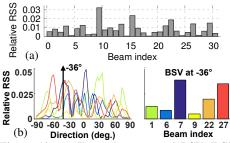
Figure 10: (a) Example measured BSV (RSS across all beam patterns for a given angle.) (b) Derive BSV from beam patterns at -36°.
