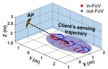
Figure 9: AP-pose sensing: Determine the orientation from a 3D ellipsoid that covers all client's poses in the AP's FoV.
