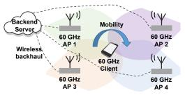
Figure 1: Multi-AP networks: APs are partially overlapped and connected to a backend server via wireless backhaul.
