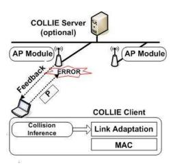
Fig. 2. Design of our COLLIE system which consists of three modules — the client which implements a majority of the logic, the AP which performs minimal packet relaying and an optional backend server (for some specific multi-AP extensions).
