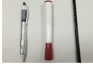
Figure 15: mmWave testbed. Testing metal-surfaced pen, plastic marker, wood pencil. Radios are placed 10cm beside 50cm×50cm writing region.
