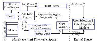
Figure 9: Firmware-kernel interaction architecture.
