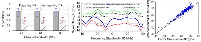
**Figure 6:** Evaluating the factors of muSINR. (a) V correlation for thrashing/no thrashing cases. (b) An example of interference estimation using V matrix. (c) Factor  $||D_k||^2/N$  at the user and AP sides.
