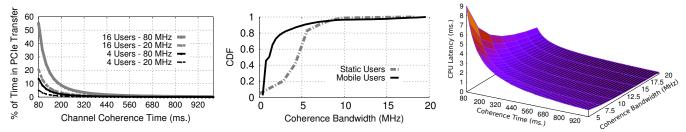
Figure 10: MUSE implementation optimizations. (a) Percentage of channel coherence time spent in PCIe (DMA) transfer. (b) Distribution of coherence bandwidth. (c) CPU execution latency for varying coherence bandwidth and time.
