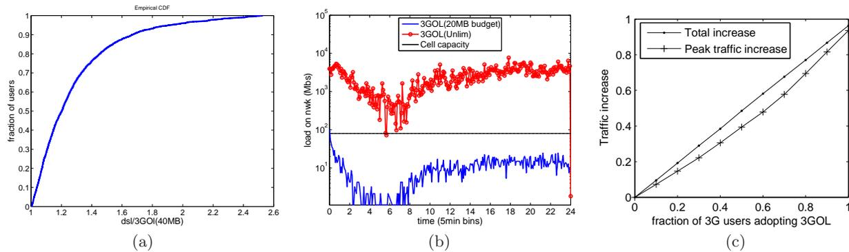
**Figure 11: CDFs of improvement of 3GOL in terms of latency per video: (a) budgeted with 40 MB daily allowance, (b) Load on cellular network by using 3GOL (budgeted) and 3GOL (unbudgeted). Y-Axis is logscale. Solid horizontal line is total backhaul capacity ( $2 \times 40$  Mbps), (c) Relative 3G traffic (total and peak-hour) increase due to 3GOL as a function of the fraction of users adopting 3GOL.**
