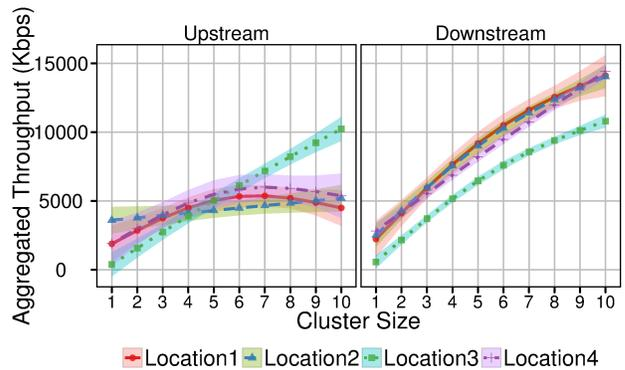
**Figure 3: Aggregated throughput (uplink and downlink) for up to ten devices.**
