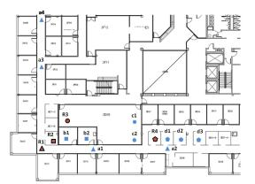
Fig. 2. Indoor Testbed; R1-R4: receivers, a1-d3: transmitters.
