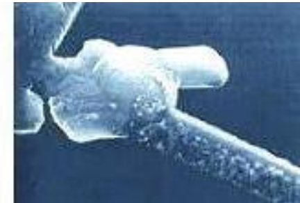
Photos of metal lines that have developed voids (above) and hillocks (below) due to electromigration. (source: www.nd.edu )
