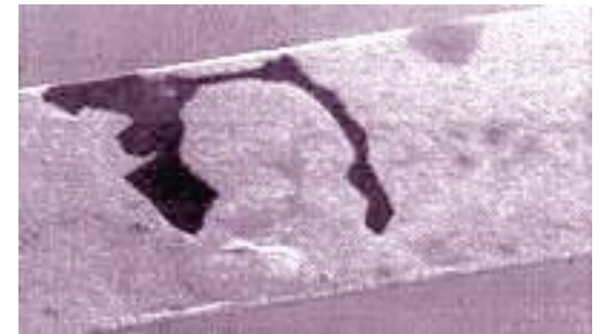
Photos of metal lines that have developed voids (above) and hillocks (below) due to electromigration. (source: www.nd.edu )
