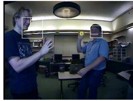
Figure 2: The visual processing step finds faces, their orientation (indicated by the small vertical or horizontal lines), and the ball (center-right).
