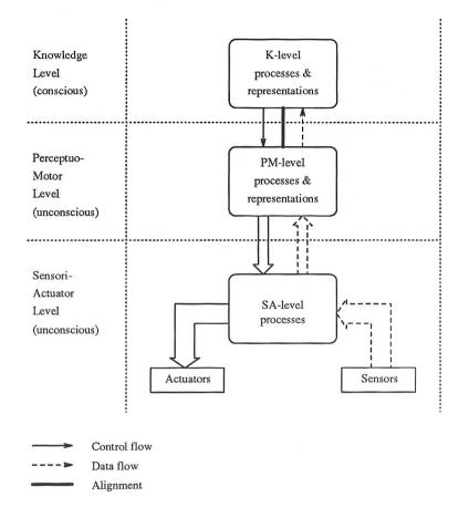
Figure 1: Schematic representation of the agent architecture. Width of control and data paths suggests the amount of information passing through (bandwidth). Sensors include both world-sensors and proprio-sensors.
