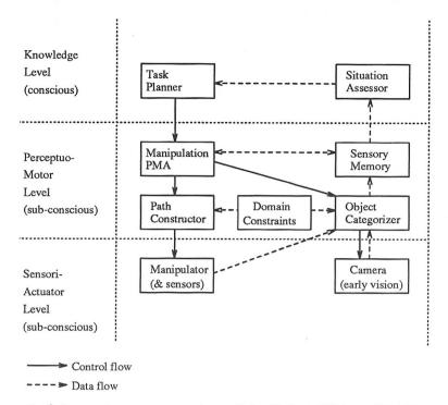
Figure 3: Schematic representation of the Robot Waiter GLAIR-agent.
