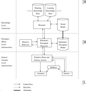
Figure 2: Schematic representation of the structure of a prototypical GLAIR-agent, an agent conforming to the GLAIR architecture.
