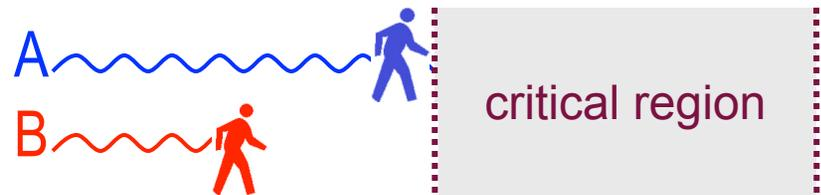
2. thread A enters CR first, preventing B from entering (B is waiting or is blocked)
