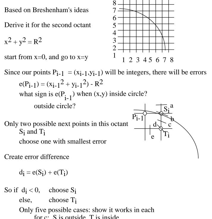
Only five possible cases: show it works in each for c: S is outside, T is inside errors will have opposite signs, S's positive if d < 0, T's is larger, choose S for a and b: S is on or inside circle, T inside T's is negative, S's is negative or 0 d < 0, choose S for d and e: T is on or outside; S is outside S's error positive, T's is positive d > 0, choose T CSE 480/580 Lecture 7
