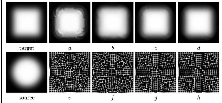
**Fig. 1.** Influence of the kernel size on the registration smoothness. Images *a*, *b*, *c* and *d* are the result images from the registration of the source image into the target image using the F3D with a Gaussian kernel radius of 1, 2, 3 and 4 respectively. Images *e*, *f*, *g* and *h* are the resulting deformation fields and are displayed with the same organisation.
