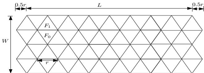
Fig. 1. Segmentation of the field into equilateral triangles
