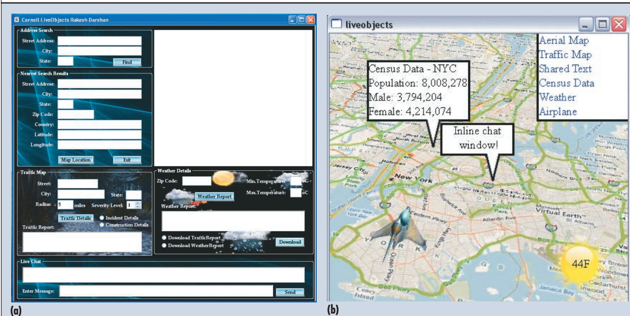
Figure 1. Example service-oriented computing application using (a) a minibrowser-style mashup and (b) Live Distributed Objects.
