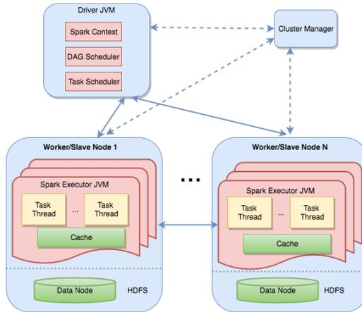
Figure 1: Spark Architecture
