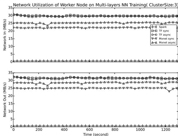
Figure 11: Network Utilization of Multi-layers NN Training on the Three Systems, Cluster size =3 (3 workers +1 ps)
