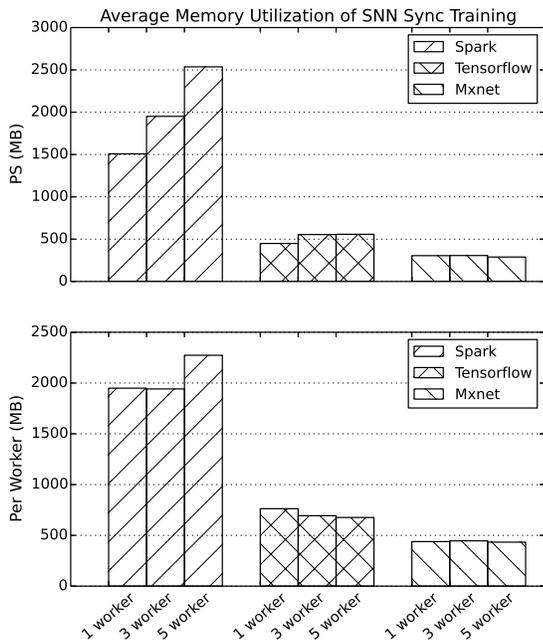
Figure 14: Average Memory Utilization with Different Cluster Size
