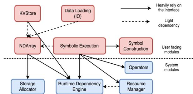
Figure 6: MXNet Components
