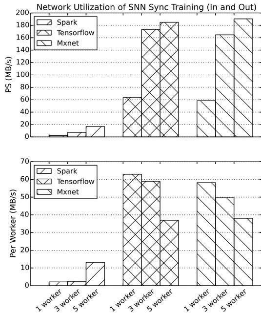
Figure 15: Average Network Utilization with Different Cluster Size
