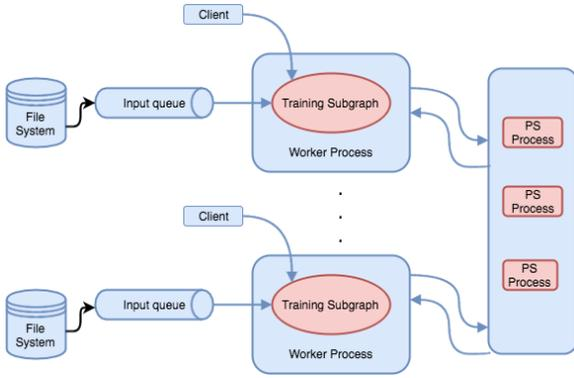
Figure 4: TensorFlow Between-Graph Replicated Training
