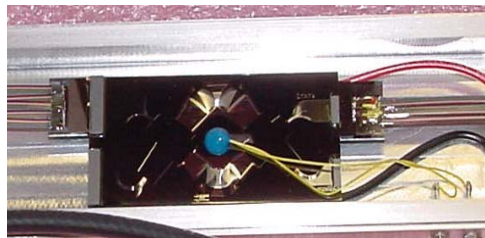
40 channels packaged device Dimensions: 5 x 2.5 cm 2
