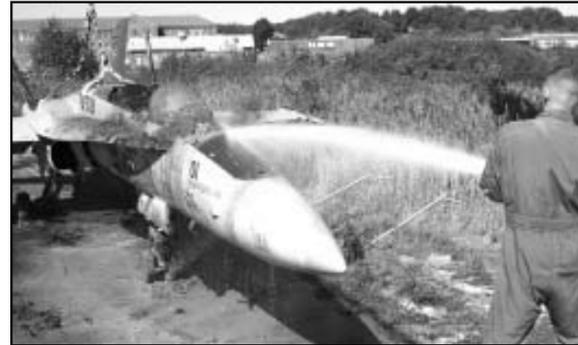
A Marine washes down an F/A-18A Hornet recovered from a marsh after brakes on the fighter jet failed during touch-and-go landings at the Quantico Marine Corps Air Facility in Quantico, Va.
