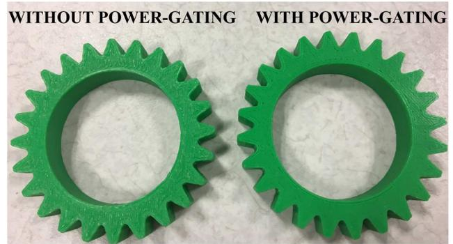
Figure 17: Comparison of printing quality. No any significant visual differences can be observed.
