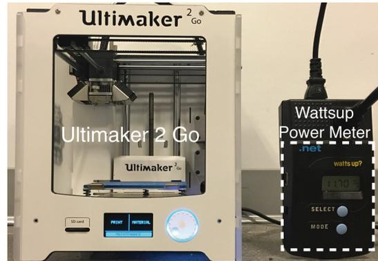
Figure 3: Experimental setup for power measurement. A WattsUp power meter connected in series to a power line and a 3D printer.
