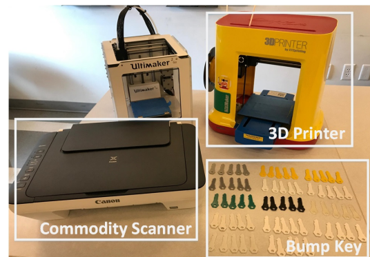
Figure 9: Experimental setup for 3D printer identification where bump keys are fabricated and scanned via a commodity scanner.
