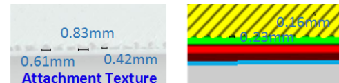
(b) Near the object's edge, the width and shape of clearances are different from the design model.
