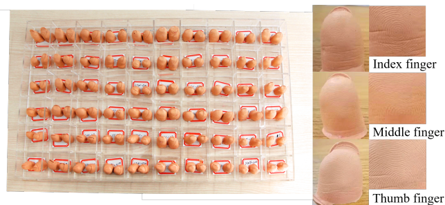
Fig. 3. An array of high-precision fake fingers modeled from index, middle and thumb fingers from 20 subjects.
