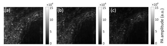
Fig. 8. Comparison of different excitation powers. (a) PA result acquired with 800mJ/pulse laser power. (b) PA result acquired with 650mJ/pulse laser power. (c) PA result acquired with 475mJ/pulse laser power. These three images are plotted using the same colorbar.
