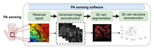
Fig. 4. PAvessel software scheme illustration.
