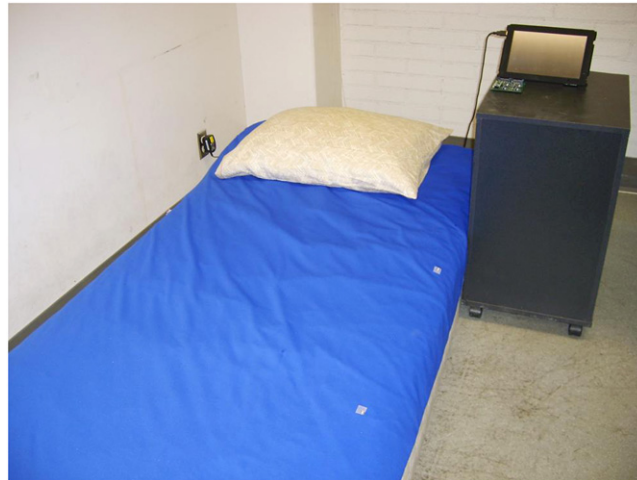
Fig. 2. Pressure sensitive bedsheet.
