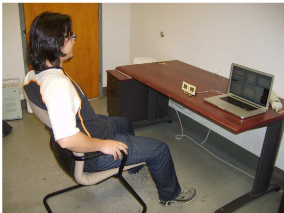
Fig. 11. The Doppler radar is measuring vital signs from one subject.
