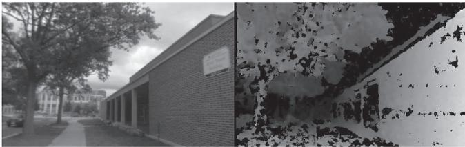
Figure 2: A typical image with its disparity map. Invalid regions of the disparity map are in black.
