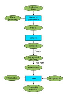
Figure 1. DsmSim Build Process for the Intel Architecture.
