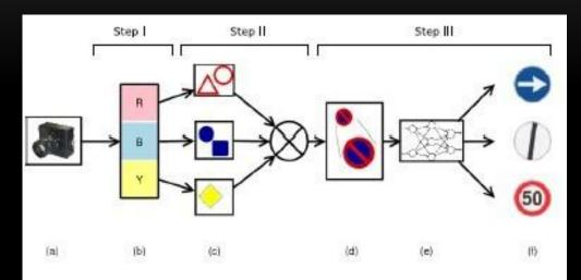
Fig. 1. Algorithm flowchart, (a) Image acquisition; (b) color segmentation; (c) shape detection; (d) bounding box scaling; (e) classification; (f) output.
