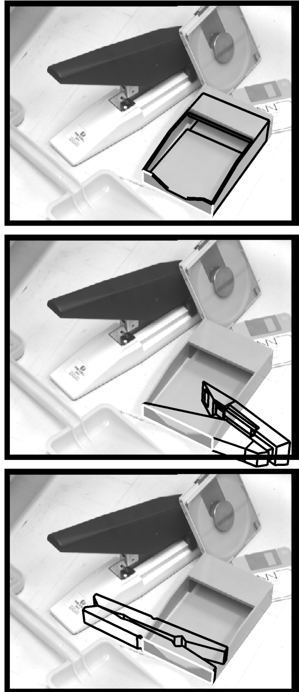
Fig. 1. A single image grouping (white lines) indicates several possible model matches (black lines) via indexing. At most, one of these may be valid.
