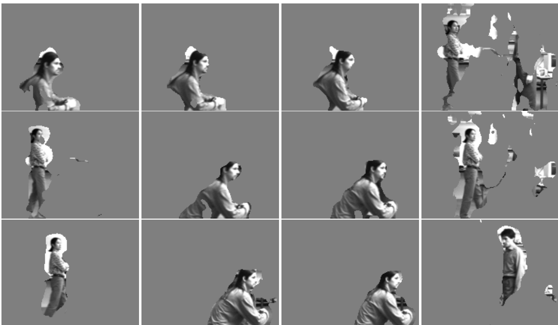
Figure 17: Target masks computed for the sequence in Figure 16. Top-left to bottom-right. Every 5th frame is shown (40 msec between frames).
