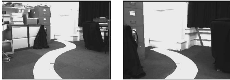
Figure 7: Two examples of the most distant visible tangent point detected and fixated in views from the robot's camera.
