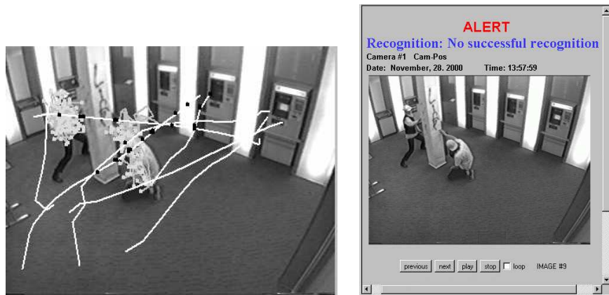
Figure 9. Detection of an unusual motion event caused by rapid movements of an act of vandalism.
