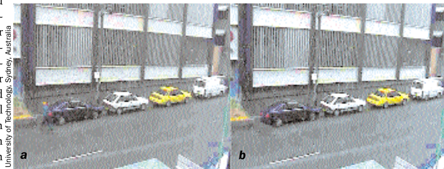
Figure 3. This parking-lot surveillance system subtracts the static background image, distinguishes a person from moving vehicles, locates the head, and calculates the speed of the head in each frame.
