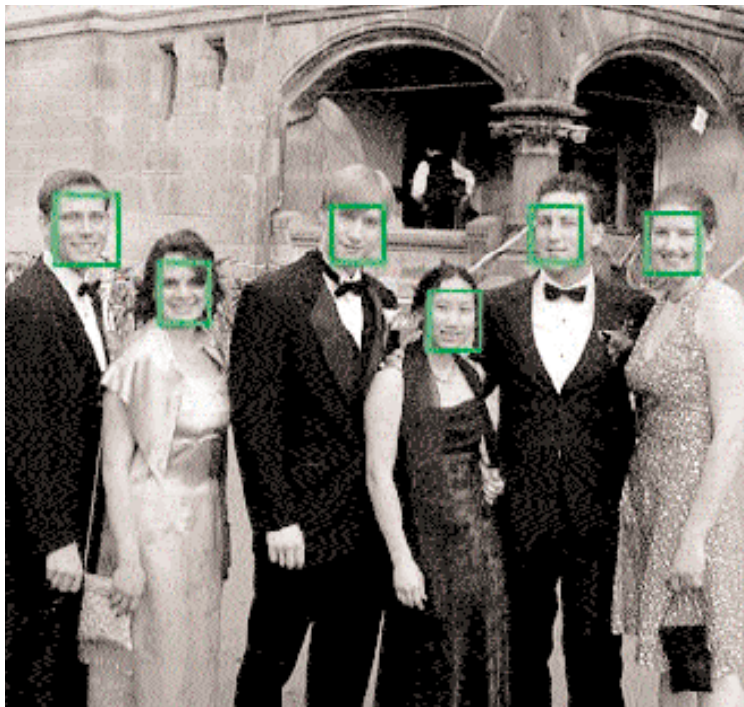
Figure 1. The Face Detection Project can automatically distinguish images containing faces from other images and put a box around each detected face—frontal, profile, or three-quarter images.
