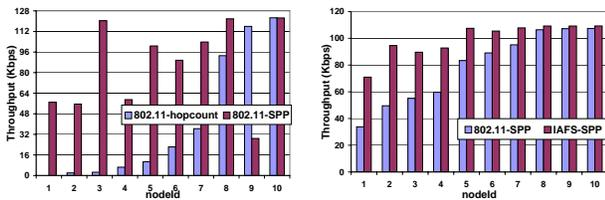
Fig. 1. Throughput comparison of two multicast trees with 10 multicast members in a 50-node WMN. (a) a hop-count and an SPP-based tree both using 802.11. The source sending rate is 128Kbps. (b) two SPP-based trees using 802.11 and IAFS. The source sending rate is based on the cycle length of IAFS’s computed schedule.
