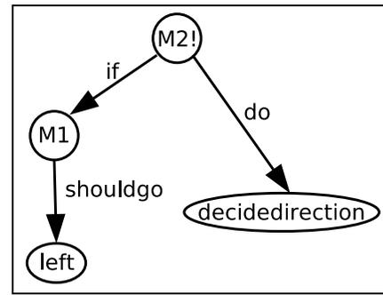
Figure 1: M1: `shouldgo(left)`: The proposition that the robot should go left; M2: `ifdo(shouldgo(left), decidedirection)`: the policy that in order to determine whether the robot should go left, the robot should perform a `decidedirection` action
