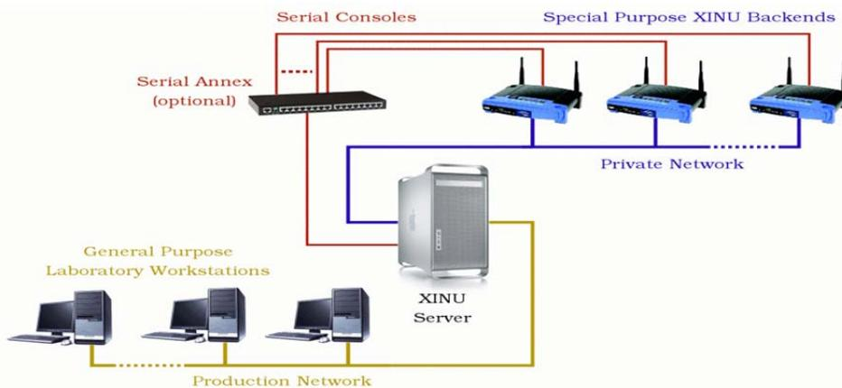
Figure 2 Expanded NEXOS environment with a central server
