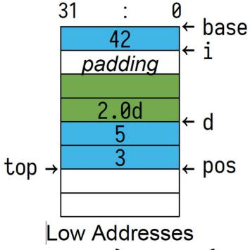
push struct { int x; int y; } pos = { x = 3, y = 5 }; Stack items are typically referenced with respect to its top. E.g., d is at top + 8
