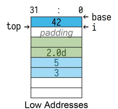
pop 20 bytes to remove pos and d Note that the unused data remains present on the stack.
