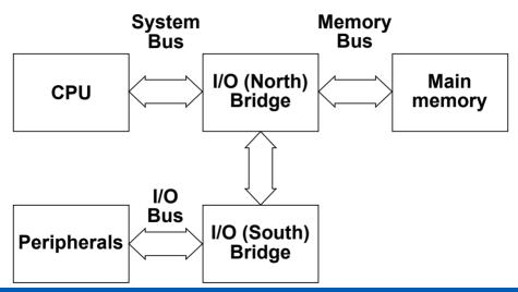
A bus has a width, which is literally the number of wires it has.<sup>¶</sup>
