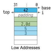
pop 20 bytes to remove pos and d Note that the unused data remains present on the stack.
