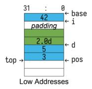
Stack items are typically referenced with respect to its top. E.g., d is at top + 8
