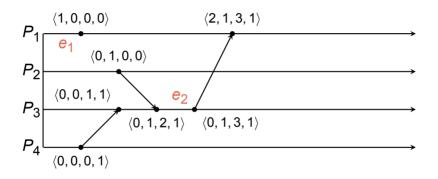
$\begin{array}{l} \textbf{e_1} \text{ is unambiguously concurrent with } \textbf{e_2} \\ \text{because } \langle 1,0,0,0\rangle \parallel \langle 0,1,3,1\rangle \end{array}$
