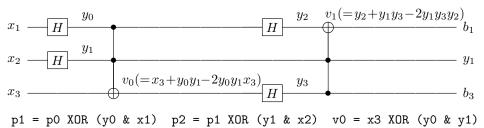
$p3 = p2 \text{ XOR } (y2 \& y0) \quad p4 = p3 \text{ XOR } (y3 \& v0) \quad v1 = y2 \text{ XOR } (y3 \& y1)$
