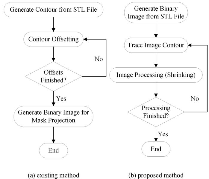
FIGURE 1. Flow Chart of Slicing and Tool Path Planning for Hybrid SLA.
