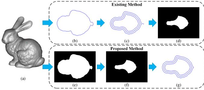
**FIGURE 2.** Bunny Model: (a) original 3D model, (b) original contour, (c) offset contours, (d) mask image, (e) original image, (f) shrunken image, (g) reconstructed contours.
